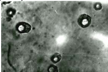
Fig.2 Primary gas-liquid inclusions in quartz of Donets Basin sandstones, 250 x magnification
