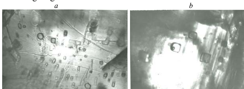
Fig 1. Gas-liquid inclusions in the salts of Ayrshagyl deposit a and Tyulyus deposit b , 250 x magnification
