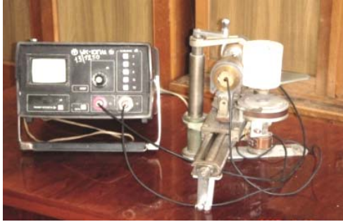
Fig. 1 - General view of the stand to determine the propagation velocity of longitudinal and transverse waves with an assembly module for positioning a rock sample with sensors
