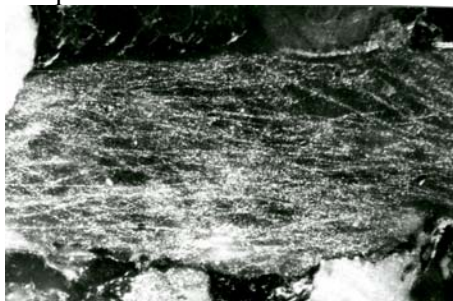
Fig. 3 Quartz grain with Boehm stripes, carboniferous sandstone of Donets Basin, oblique illumination method, 100 X magnification
