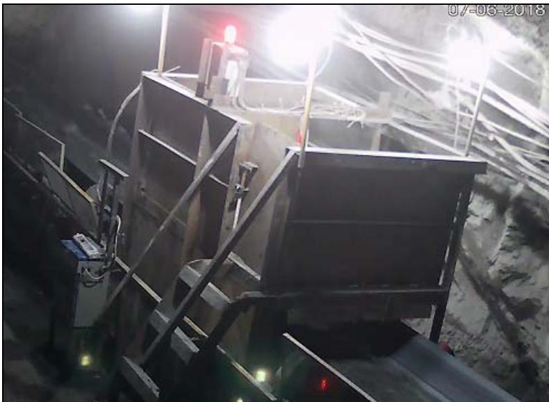
Fig. 7. – RCS on the conveyor in Nurkazgan underground mine
