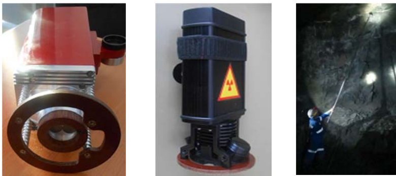
Fig. 2. RPP-12 and RPP-12RI spectrometers
